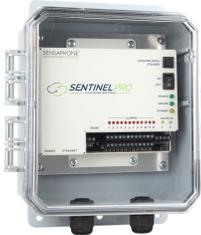
The Sentinel PRO system monitors, delivers alarms and logs data input/output points from third-party Modbus sensors, transducers and PLCs. It supports Modbus RTU/485 and Modbus TCP. The system interacts with all existing sensors within a facility and provides operators with on-demand live status and data acquisition from any internet-connected device.
